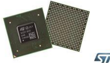
STiD337 DVB-S2/S2X satellite demodulator
